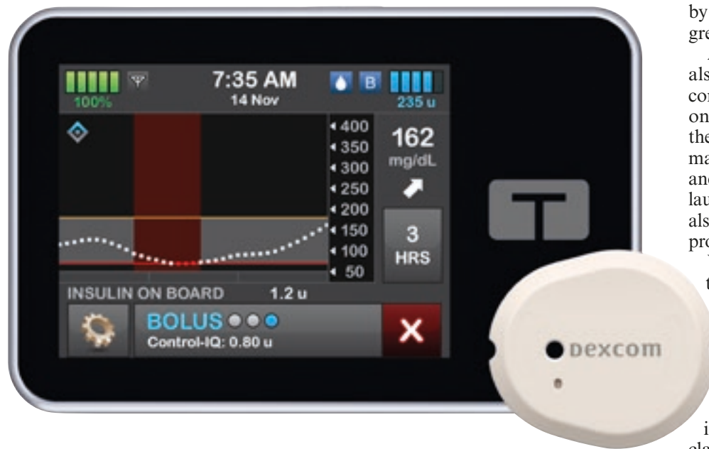
The Dexcom G7 Continuous Glucose Monitor (CGM) wearable sensor will connect with the t:slim X2 insulin pump from Tandem. Photo courtesy Dexcom
